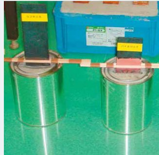
Specimens embedded in mortar
