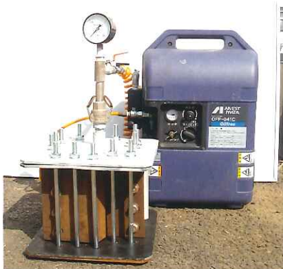
Photograph-10. Watertightness pressure test system. Chart-3. The pressure water tank unit which a steel sheet-pile tab was set on.
